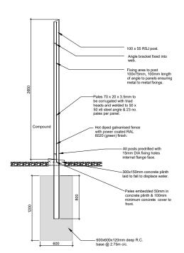
Typical palisade fencing details - section
