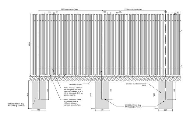
Typical palisade fencing details - elevation
